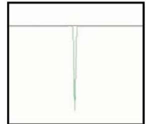
PST failed, valve is stuck.
