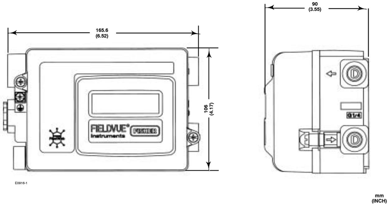
Figure 4. Dimensions for Type DVC2000 Digital Valve Controller
