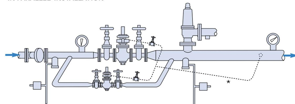
\*Balance lines are only required on some steam applications, they are not required on air/gas applications.
