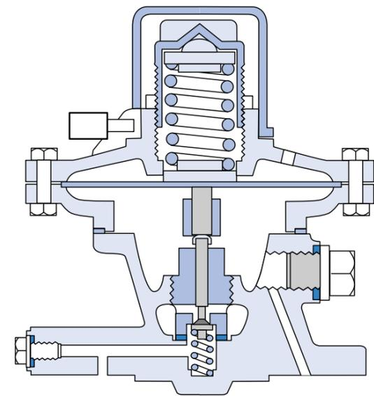
The standard 'G4' pilot top can reduce pressures down to 0.35 Barg (5 Psig). For pressures below this, a bronze low pressure pilot top can be fitted in place of the standard top. It is suitable for outlet pressures from 0.07 to 0.35 Barg (1 to 5 Psig) using the yellow spring. The low pressure top is available for fitting on to valve sizes 15 to 100mm (1/2 to 4 inch), and a balance line should always be fitted to a low pressure top, on steam duty and never on gas duty.
