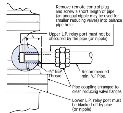
'A' dimension must be  $1\frac{5}{16} \pm 1/16$ " on all stainless steel valves or CS Fig 2046. All other valves with bronze pilot tops, the pipe should penetrate 1" minimum.
